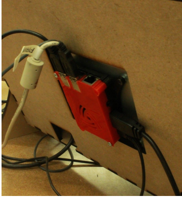
They have Raspberry Pi computers on the back, in 3D printed cases, running ChiliPi-Kiosk.
